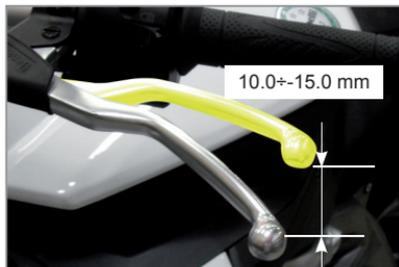
Check the clutch lever backlash regularly and adjust as necessary.
